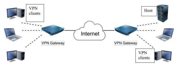
*Figure 2.6: Example of Gateway-to-gateway VPN architecture* (Barker *et al.*, 2020, p. 12)
