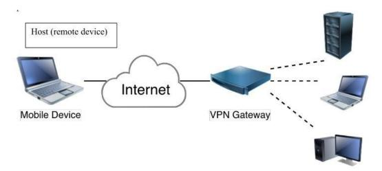
*Figure 2.7: Example of remote access VPN architecture* (Barker *et al.*, 2020, p. 13)
